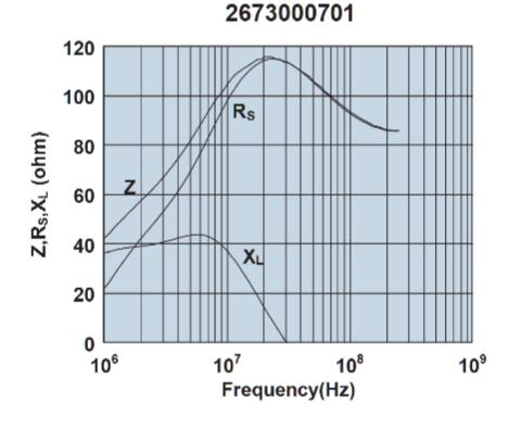
Impedance, reactance, and resistance vs. frequency.
