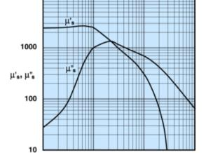
Measured on a 2673000301 bead using the HP 4284A and the HP 4291A.
